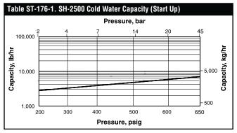
Note: Cold water capacity for start-up loads only. When superheat present, there will be minimal condensate.
