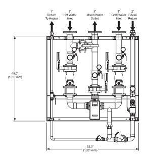
\*DMC50 is a DMC80 supplied with a 2" pipe work, fittings with union inlet/outlet connections.
